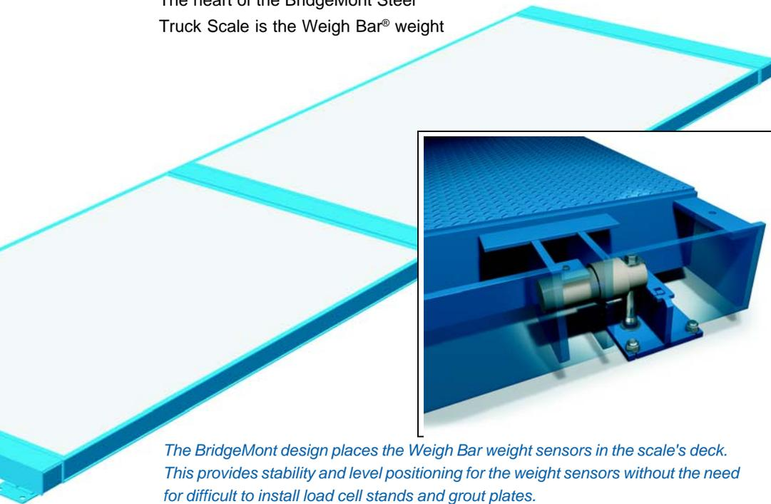
*The BridgeMont design places the Weigh Bar weight sensors in the scale's deck. This provides stability and level positioning for the weight sensors without the need for difficult to install load cell stands and grout plates.*
